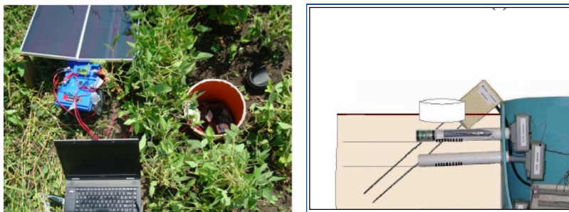
Fig. 3. Overview and section of the monitoring system of CO 2 , O 2 , moisture and temperature in the soil, based on the gradient method [28]
