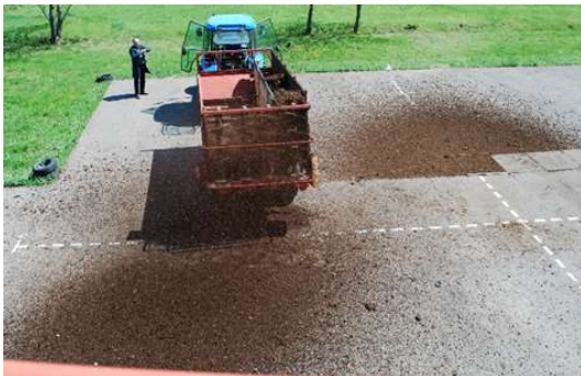
Fig.3. Compost distribution on concrete platform
