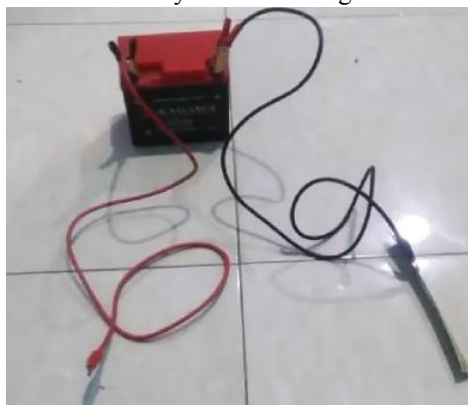
Fig. 2. Conductivity test Apparatus Setup
