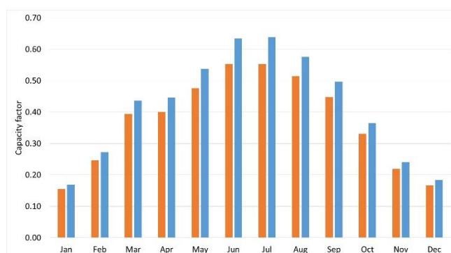
Fig.11. Computed capacity factors over the year. 10% increased solar field surface and TES increased to 10 h.
