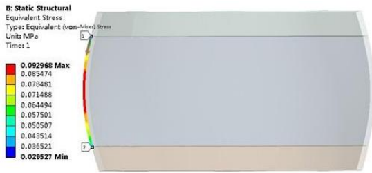
Fig. 6. Reactor winding stress at -40^{\circ}\text{C}
