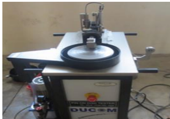
Fig 2. Pin on Disc Tribometer Used
