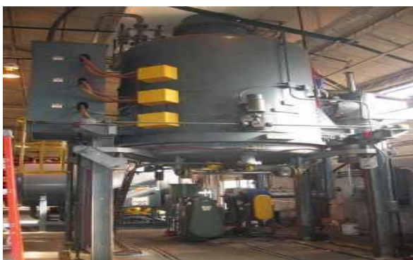
Fig 1. Plasma Nitriding Furnace Used
