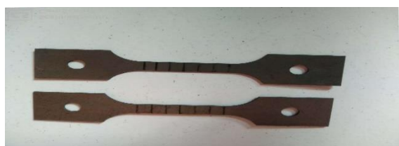
Fig 3: a) Marked Tensile Test specimen
