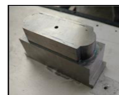
Fig.2.4. Core and cavity sub insert of DN20 vent
