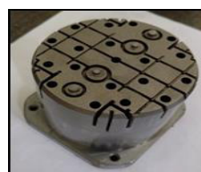
Fig.2.4. Core and cavity sub insert of DN20 vent
