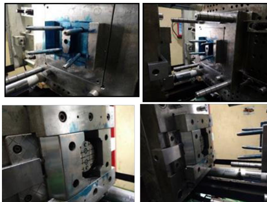
Fig.3.2. Dn20 vent mould core and cavity manufacturing process.
