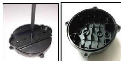
Fig.3.3. DN20 vent manufacturing (melting temperature is 300°C, mould temperature is 70°C, injection time is 0.7s.)
