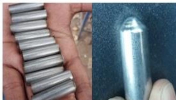
Fig. 1. AISI Austenitic stainless steel fractured into pieces and machined in bullet shape
