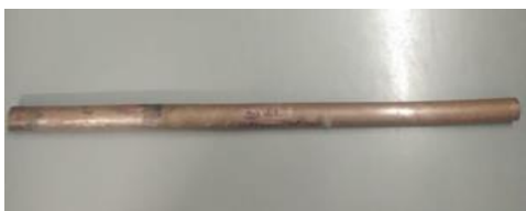
Fig 1. Copper heat pipe with meshed wick
