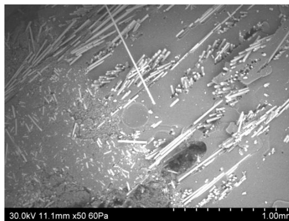
Fig. 7. SEM Images of Izod impact test specimen indicating matrix domination over fiber.
