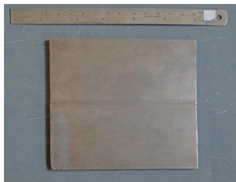
Fig. 2. Butt weld joint produced through Fiber Laser Welding
