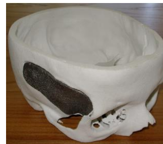
Fig. 3. Custom-made skull plate manufactured in medical-grade titanium using SLM technology [18]
