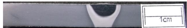
Fig. 7. Abrasive cutter cut specimens used after weld to analysis effect on Microstructure and Grain Size, Hardness, grain size.
