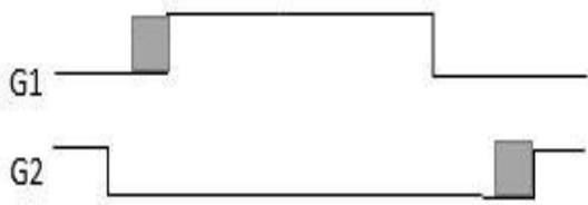
Fig.7. The Dead region from a dead-band circuit
