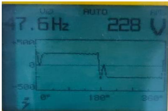
Fig.13. Hardware output voltage and frequency
