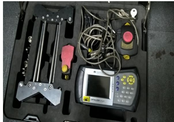
Fig. 4. Laser Shaft Alignment
