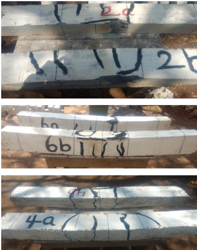
Fig3. Failure and Crack Pattern of M30 Beam
