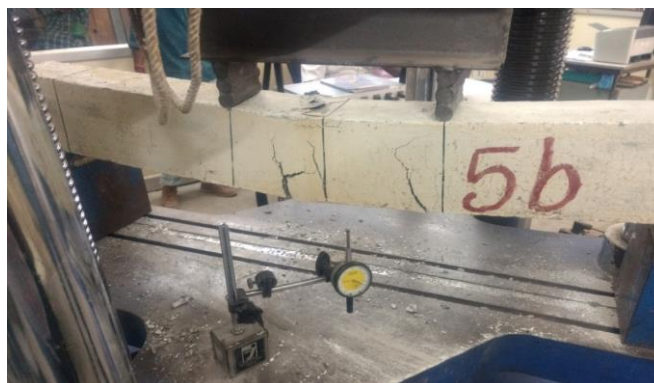
Fig 2. Flexural testing of beams
