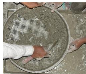
Fig. 2. Sieving of concrete through 4.75mm sieve
