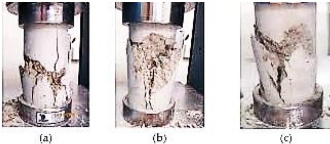
Fig. 4. Failure patterns of (a) 12 mm length + 0.4% fibre (b) 36 mm length + 0.4% fibre (c) 50 mm length + 0.3% fibre
