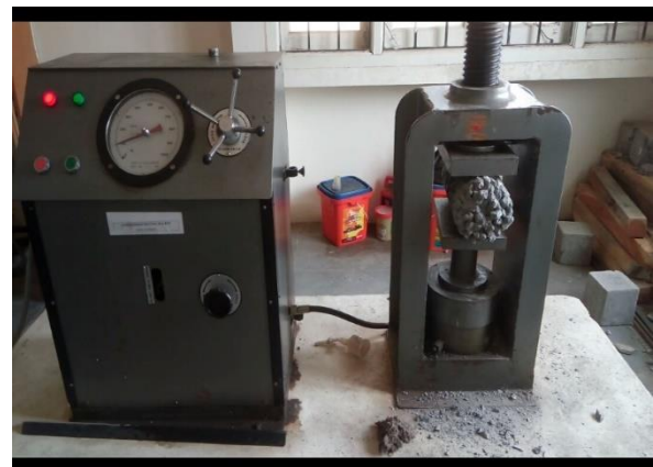
Fig. 5. Split tensile strength on Cylinder specimen
