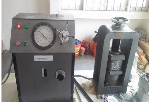
Fig. 1. Compressive strength test on cube specimen
