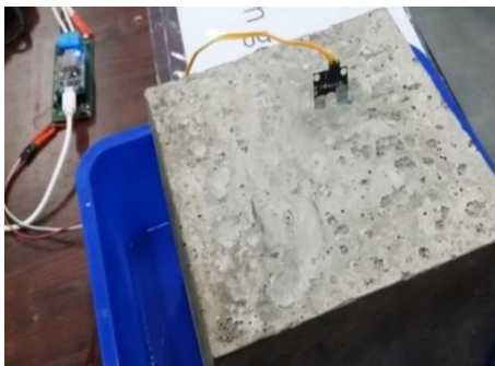
Fig. 2. Smart concrete curing
