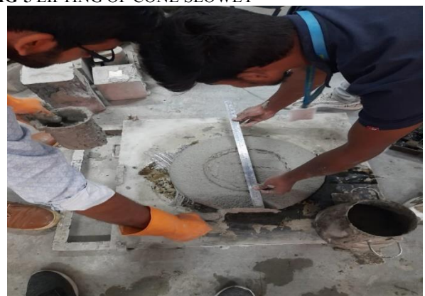
Fig. 6. MEASURING THE FLOW OF THE CONCRETE
