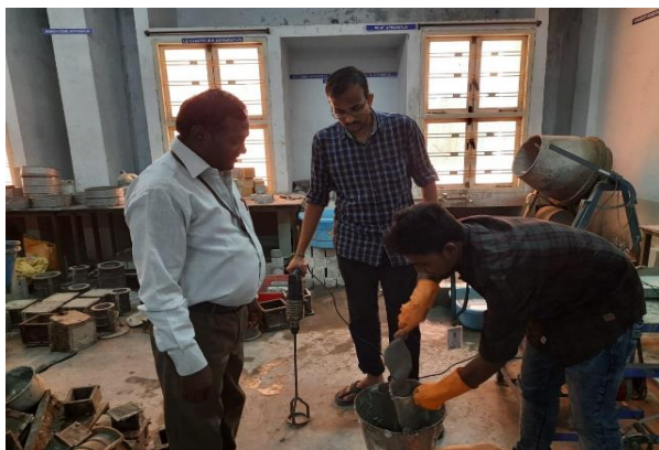
Fig. 3. MIXING OF FOAM CONCRETE
