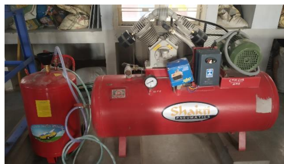
Fig. 1. FOAM GENERATOR CONNECTED TO AIR COMPRESSOR
