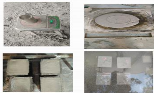
Fig. 3. Preparation of Moulds and Curing
