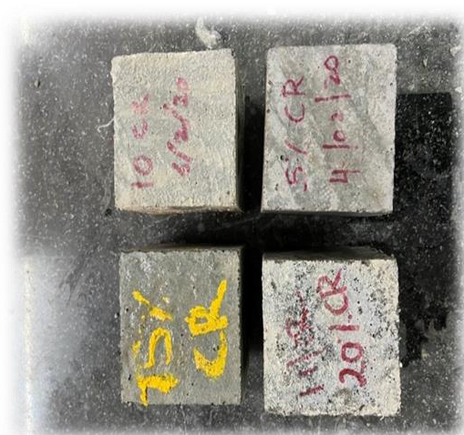
Fig.3 Different cubes with different % of crumb rubber
