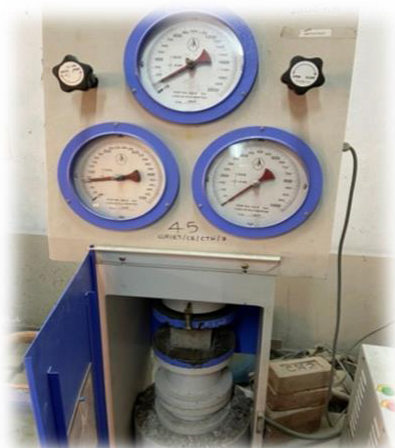
Fig.4 Testing of Compressive strength for 20% crumb rubber
