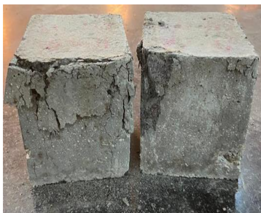
Fig.5 cubes after compressive strength test, 15% Crumb rubber
