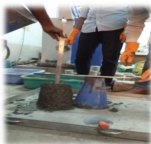
Fig.2 slump cone test for 20% crumb rubber
