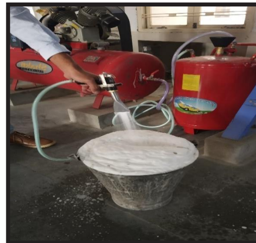
FIG-2 GENERATING FOAM FROM FOAM GENERATOR
