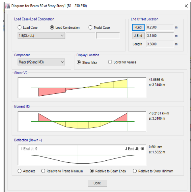
Fig.29. Maximum SF and BM of Beam B9 of conventional building
