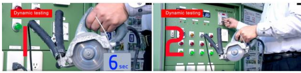
Fig. 5. Dynamic testing process of equipment power consumption.
