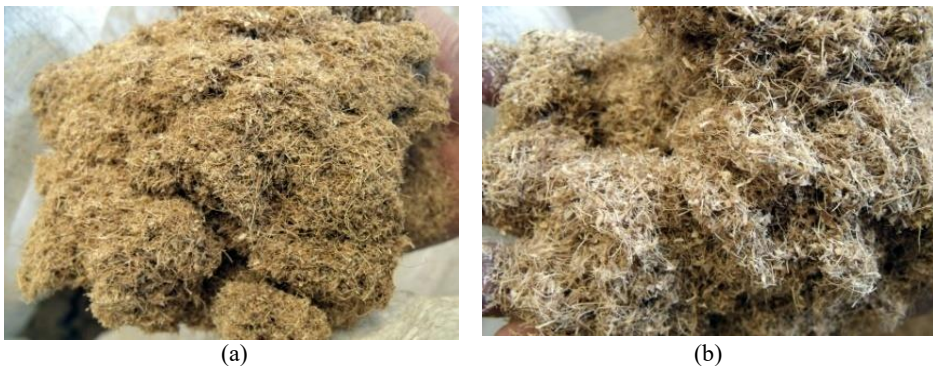
Fig. 1. The feature of bamboo shoot sheath particles with (a) 0.5-mm and (b) 0.6-mm size.
