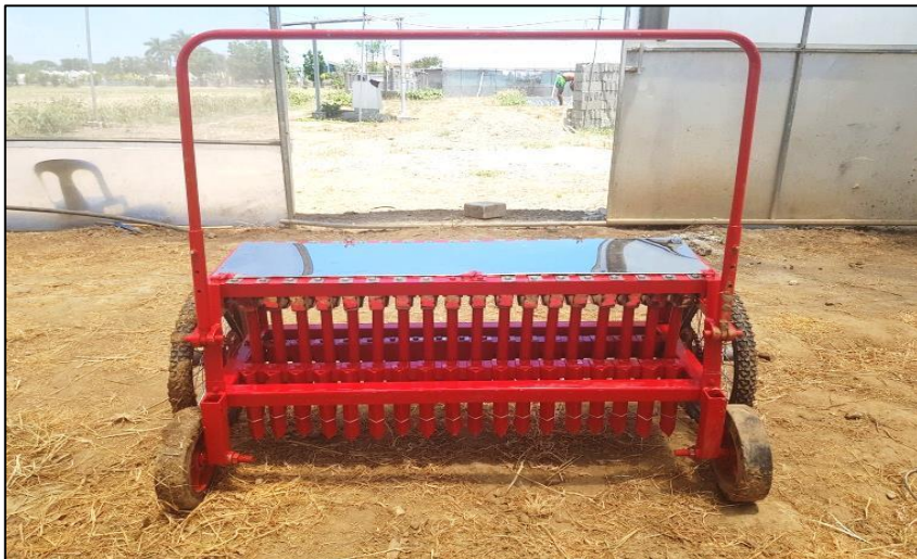
Fig. 1. Onion sowing machine for seedbed.
