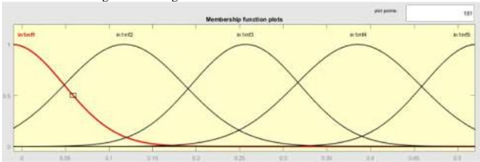
Fig. 4. Membership function of error and delta error on pitch and yaw axis.
