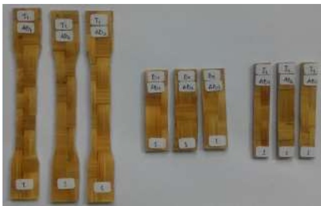
Fig. 1. Tensile, bending and impact test specimens
