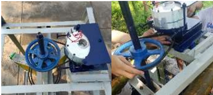
Fig 5. Pulley mechanism in system integration
