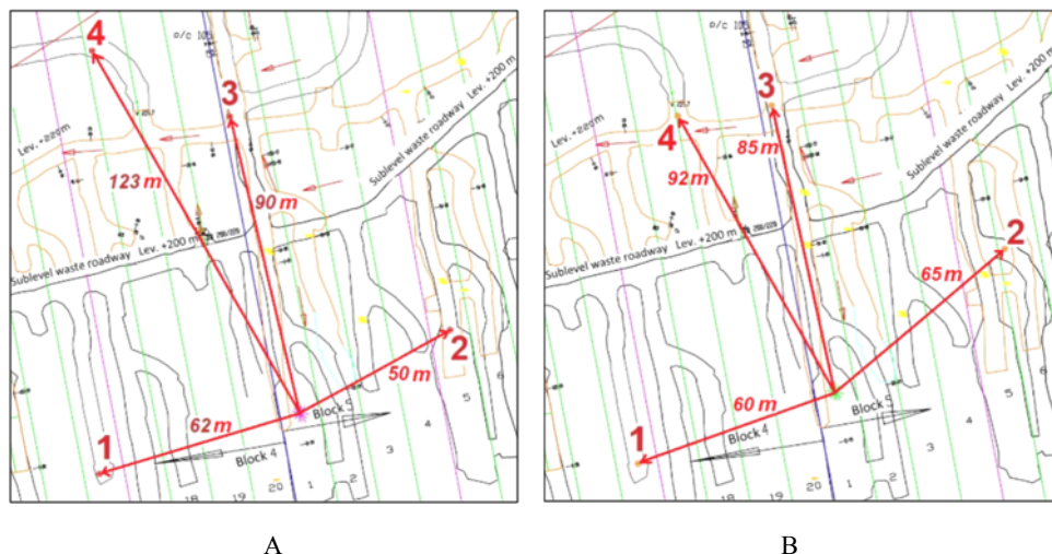
Fig. 1. Layout of measurement points on February 03 (A) and February 04 (B), 2020, and blasting points (chamber # 1, block # 5, level +220 m).
