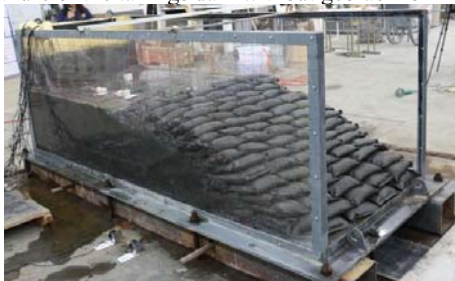
Fig.7 Failure of the tailings dam with geofabriform
