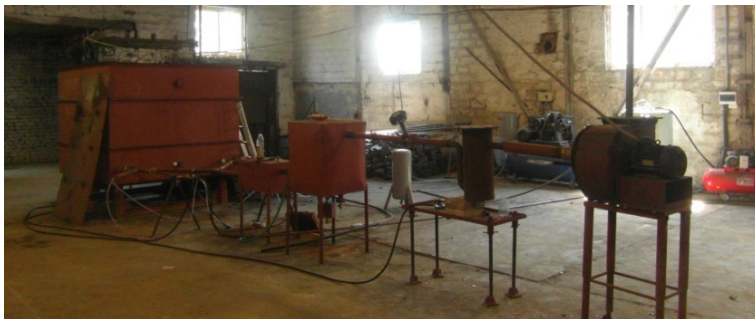
Fig. 1. Photo fixation of the laboratory setup: 1 – sectional laboratory stand, 2 – cooler tank for sampling, 3 – smoke sucker, 4 – a tank for supplying the blowing reagents; 5 – reverse T-junction; 6 – controlled blowing pipelines; 7 – blowing pipelines; 8 – pipeline for simulation of the “well-gas generator” technology; 9 – ignition channel.
