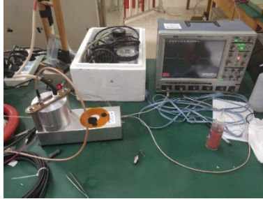
Figure 3. Space Charge Measurement System Based on Electroacoustic Pulse (PEA) Meth
