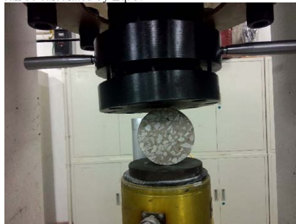
Fig. 2. Concrete disc on test by TAW-2000D Rock mechanics testing machine
