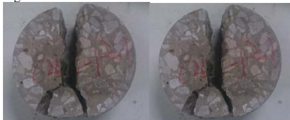
Fig. 3. Failure patterns of concrete dis with materials C25
