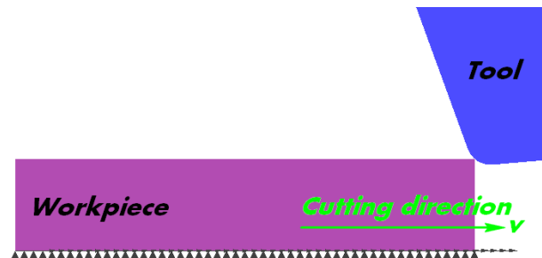
Figure 1. 2D-Orthogonal cutting FEM of the rounded-edge tool
