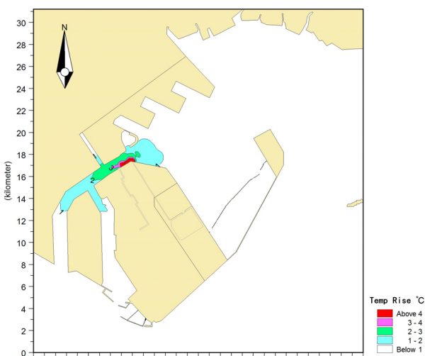
Figure 2. Envelope diagram of Maximum temperature Rise (winter)
