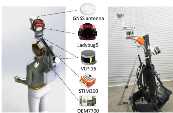
Fig. 1. Our backpack MMS system and sensors.
