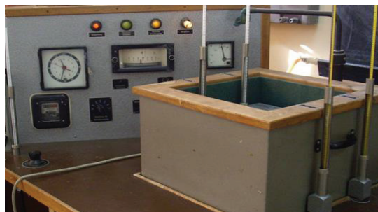
Fig. 2. Test stand based on the method of infinite flat plate
