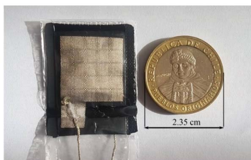
Fig. 4. Fabricated woven pressure resistive sensor [13].
