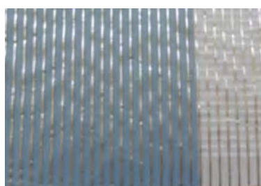
Fig. 4. Fabricated woven pressure resistive sensor [13].
