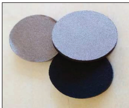
Fig. 2. Textile electrodes without edging.
