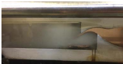
Fig. 7 Cavitator photo in a cavitation mode
