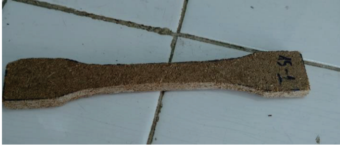
Fig. 2. Specimen of bamboo plywood tensile testing
