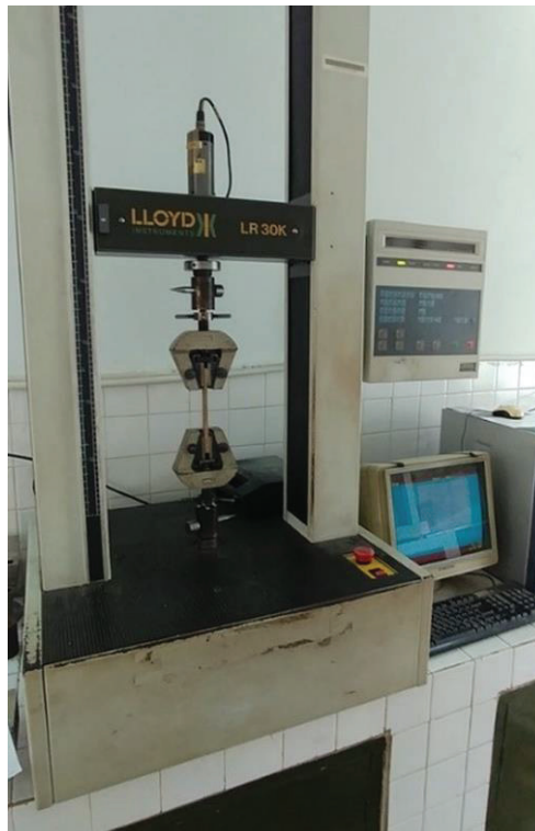
Fig. 3. Tensile testing of bamboo plywood specimen in universal tensile test machine LLOYD LR 30K
