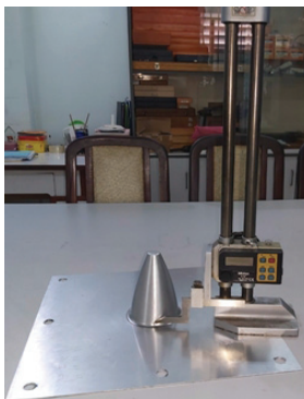
Fig.7 Measurement of mechanical failure height.
