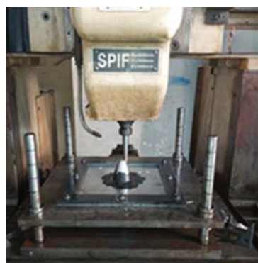
Fig.2 Practical model of Jig and TPIF process.
