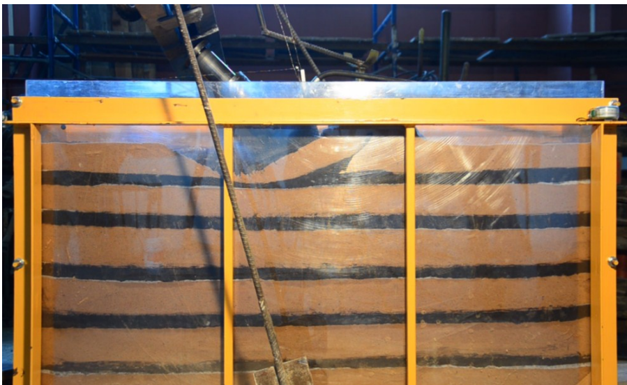
Fig.7. Loss of stability of anisotropic sandy-argillaceous base with layers of 2.5 cm.
