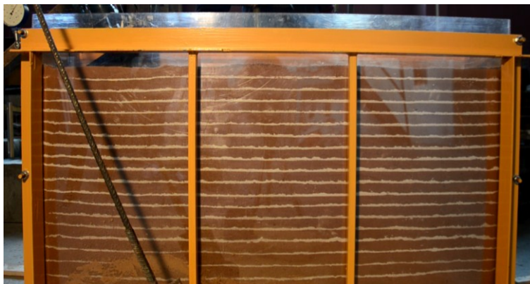
Fig.2. Uniform sandy base before testing.
