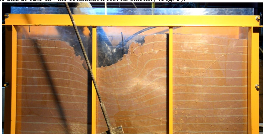
Fig.3. Loss of stability of a homogeneous sandy base.
