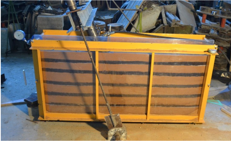
Fig.6. Anisotropic sandy-argillaceous base before testing.
