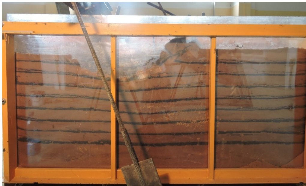
Fig.8. Loss of stability of a sandy-clay base with 0.5 cm interlayers.
