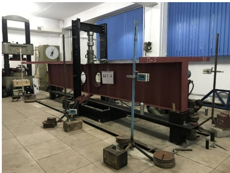
Fig. 3. General view of the installation for testing the BGS-4 beam.
