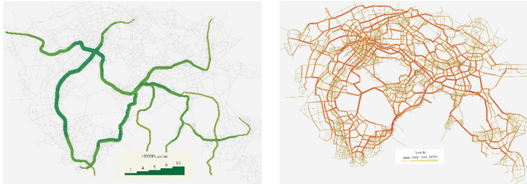
Figure 2. Distribution of rail transit passenger flow (left) and motor vehicle flow (right) in the morning peak of the future year
