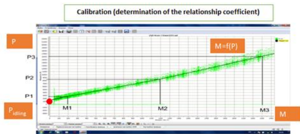
Fig.3. Determination of the relationship between torque and corrected active power.
